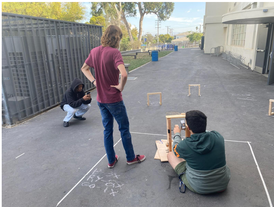
Figure 31: The device's performance is being tested in an environment that mimics the actual competition. Team members practice aiming the device toward the targets with the help of a laser pointer, and releasing the hammer so that it strikes the ball.
