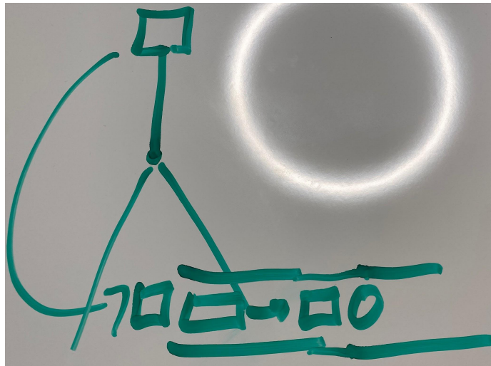
Figure 12: A hammer swings on an axle hitting a block horizontally through a rail, hitting another ball and transferring only its forward momentum.
