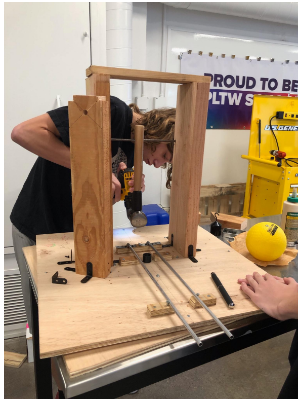
Figure 29: The second pair of vertical wooden boards is being attached to the device using L braces, screws, and a screwdriver.
