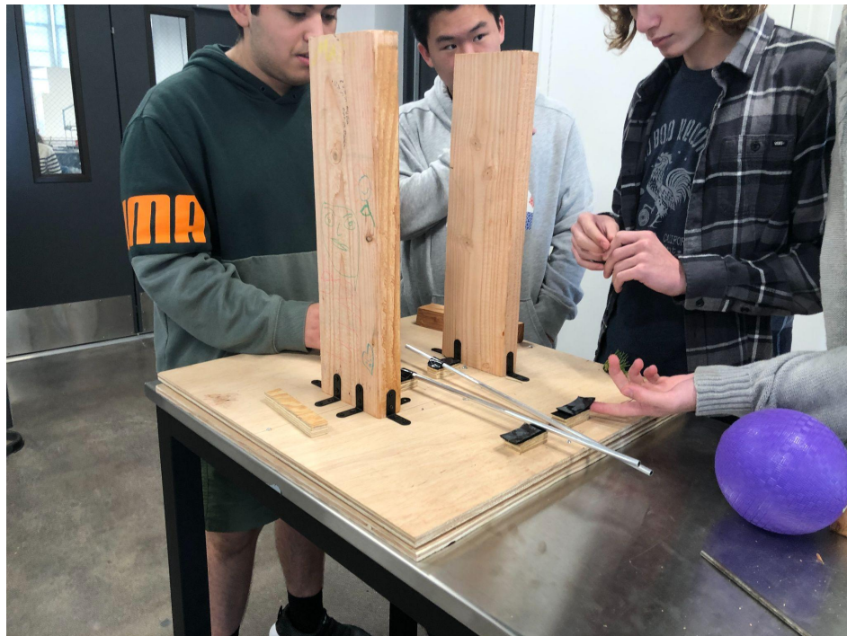
Figure 28: The device with the vertical wood boards attached to the base. The hammer has not been attached yet. Placement of the rails is being experimented with.
